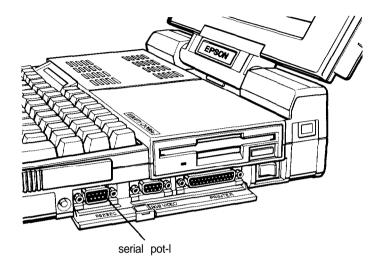
The Equity LT-286e uses an IBM PC AT-compatible, 9-pin, D-shaped male connector, so be sure you have a compatible cable or an adapting cable that converts the 9-pin output to the standard 25-pin output. To connect a serial device, follow the steps above for connecting a parallel device.
